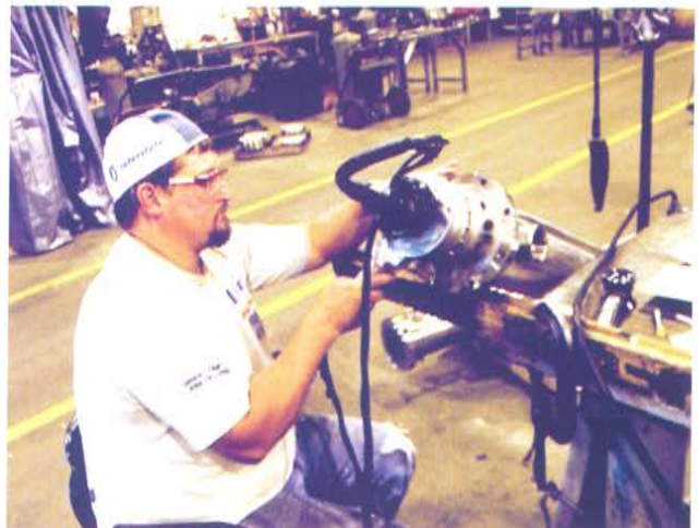
Seal-welding the tubes to the tubesheet
