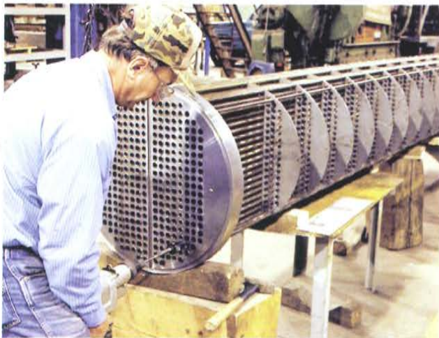
Expanding the tubes into the tubesheet
